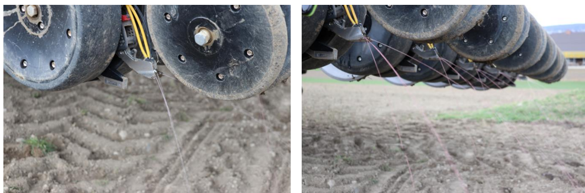
Figure 20. FurrowJet liquid fertilizer system used for planting the trial plot.
