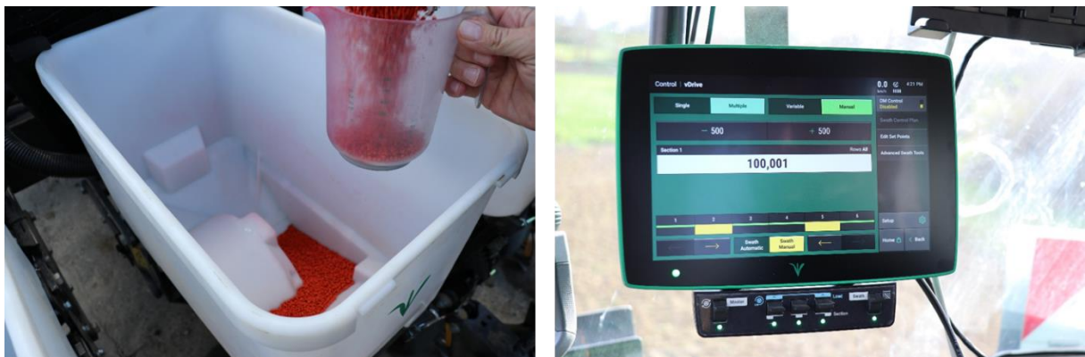
Figure 17. Sugar beet seeds (left) and 20/20 Gen3 monitor for setting the planted population (right).
