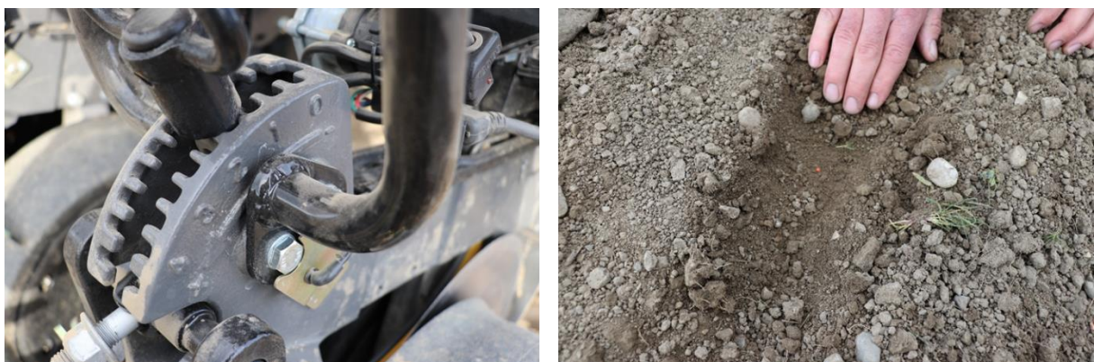
Figure 14. Planting depth setting on the planter (left) and manual check of seed placement (right).
