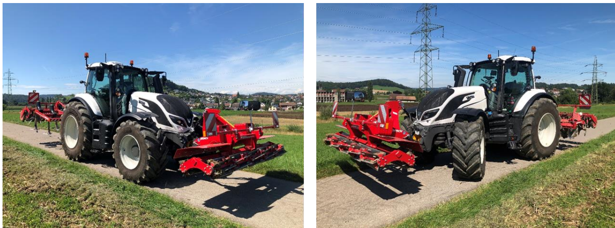
Figure 25. Combinations of knife roller and cultivator (left) and knife roller and compact disc harrow (right) used for the trial plot.
