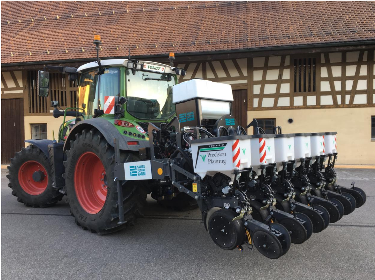
Figure 9. Precision Planting test planter with newly assembled liquid fertilizer system for sugar beet planting 2019 on the Swiss Future Farm.
