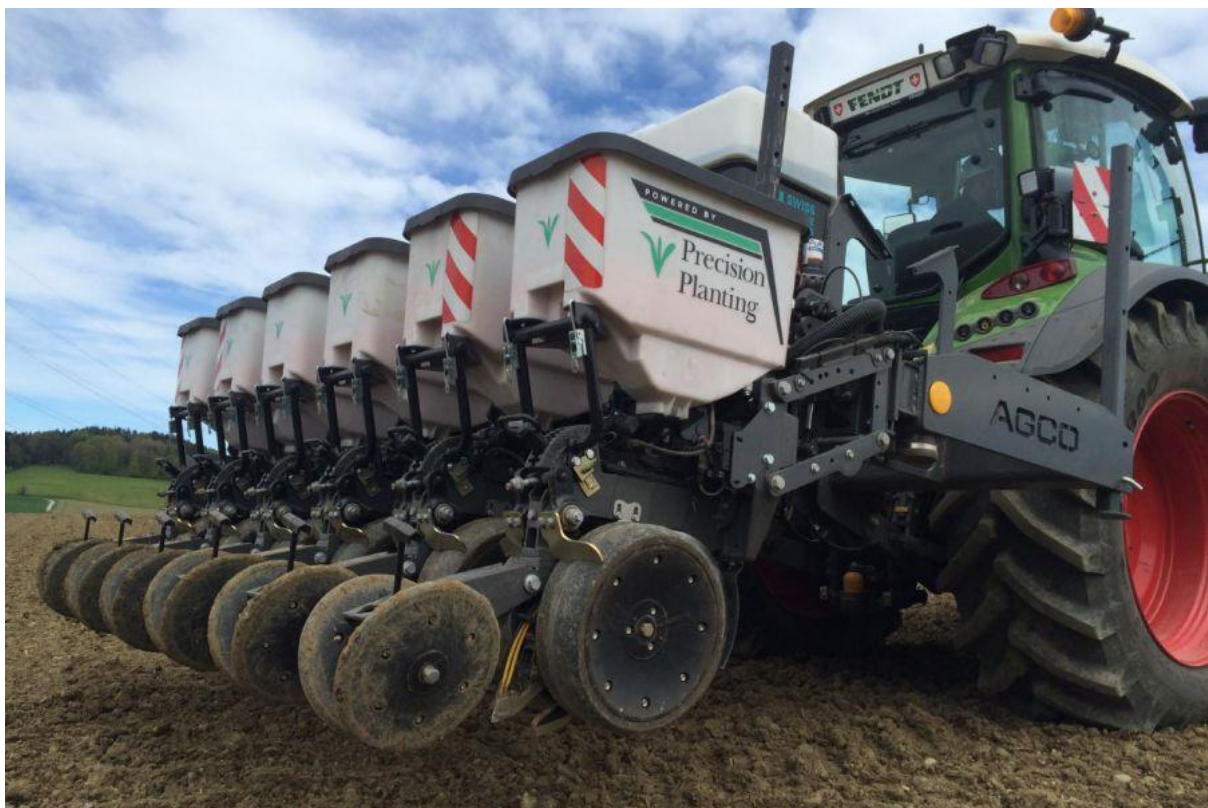
Figure 13. Precision Planting test planter with DeltaForce down force control and Fendt 516 with RTK VarioGuide, which were used for planting the trial plot.
