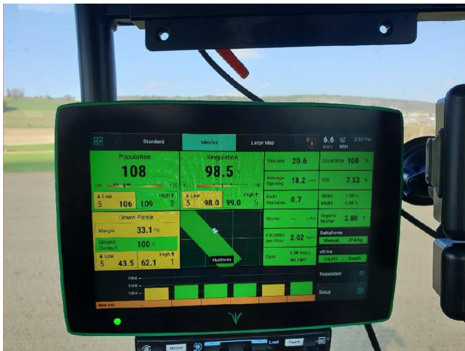
Figure 15: Precision Planting 20/20 Gen3 monitor for adjustment and control of DeltaForce down force settings during planting.
