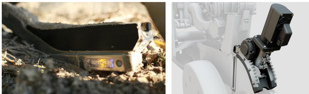
Figure 5: Precision Planting SmartFirmer for measurement of soil moisture in the furrow (left) and Precision Planting SmartDepth for real-time adaption of planting depth according to soil moisture content (right).
