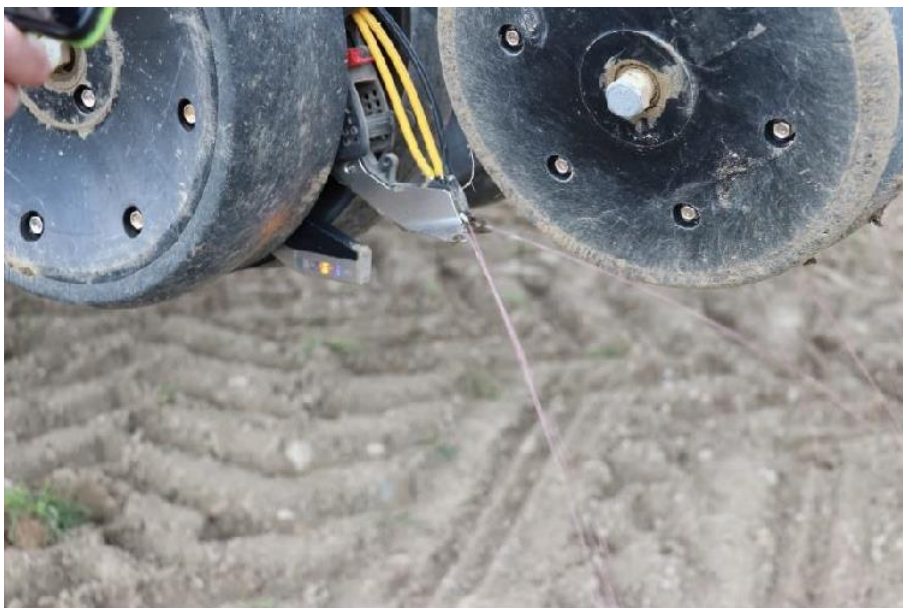
Figure 35: Precision Planting row unit equipped with FurrowJet liquid fertilizer system used for planting the trial plots.
