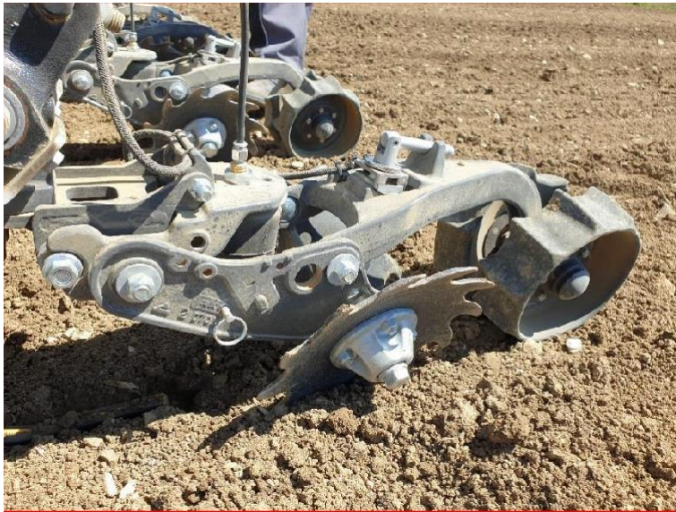
Figure 17: The pneumatic closing system Precision Planting FurrowForce enables to preserve soil moisture and to ensure yields under challenging climatic conditions.
