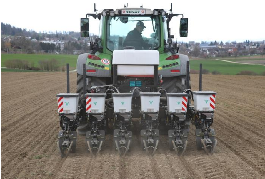
Figure 40: Precision Planting test planter equipped with DeltaForce down force control system on the trial plot.
