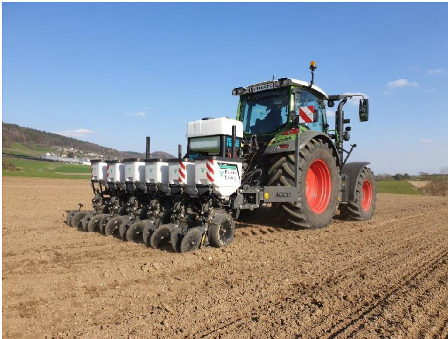
Figure 10: Precision Planting test planter equipped with FurrowJet liquid fertilizer system used for planting the trial plots.
