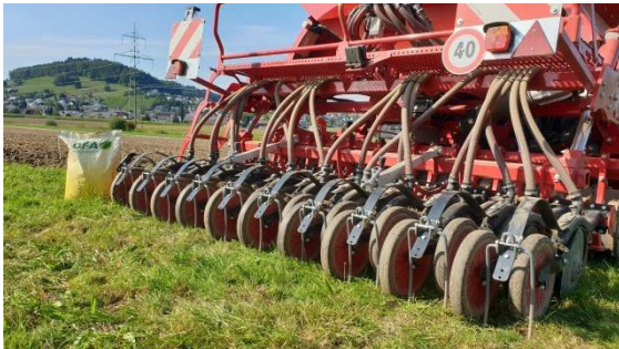
Figure 58: Horsch Express 3KR drill combination with modified arrangement of the seeding hoses from the distribution head to the seeding coulters.
