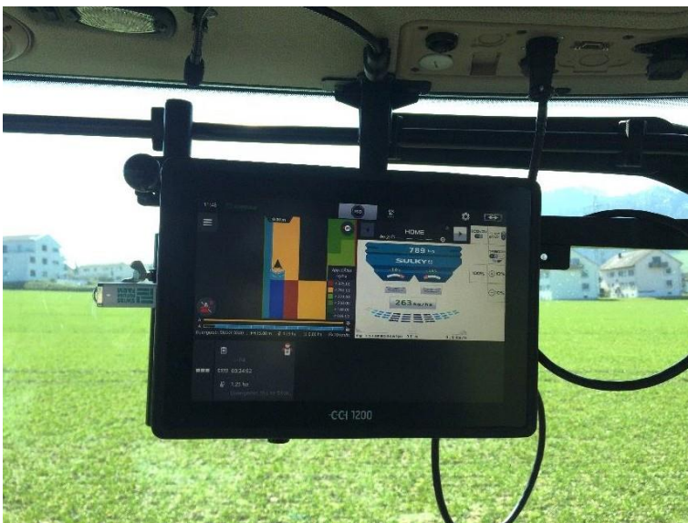
Figure 45: Universal Terminal CCI 1200 with fertilizer prescription map and ISOBUS operating mask for the fertilizer spreader.
