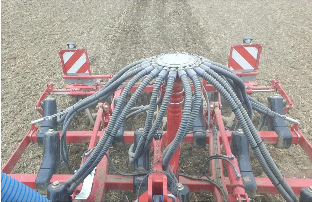
Figure 62: Distribution head of the cultivator.
