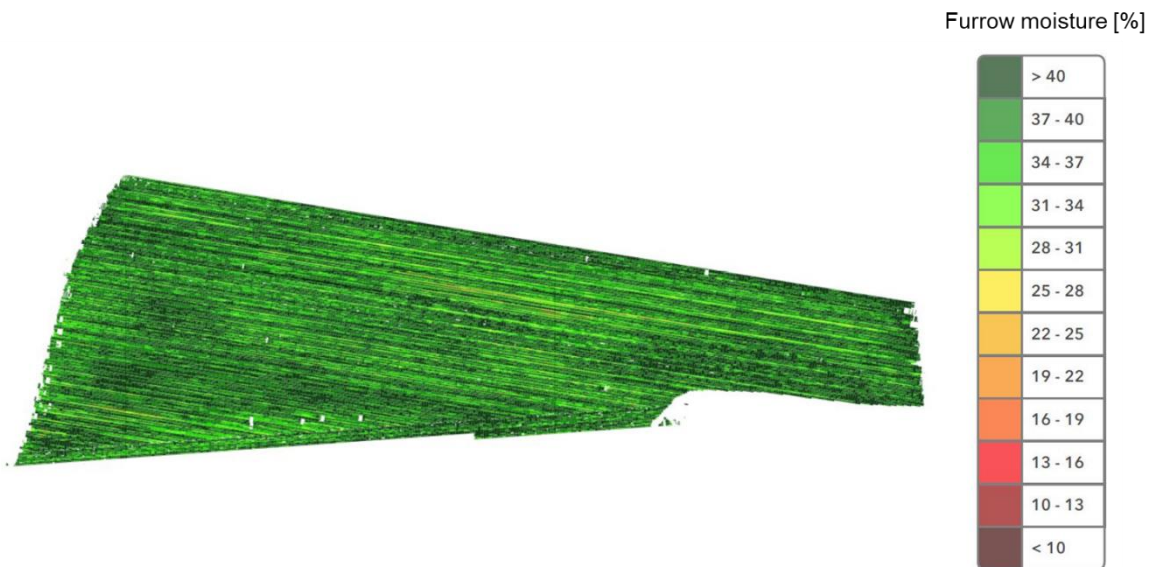
Figure 24: Furrow moisture measurement values of the SmartFirmer soil sensors during planting on the trial field of the SFF 2020 Variable Rate Study in silage corn.
