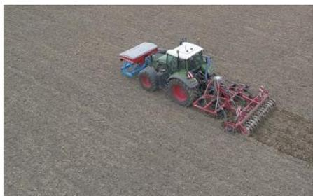
**Figure 2.** Targeted deep fertilization during tillage before rapeseed planting.
