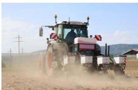
**Figure 4.** In 2020, the planting depth of 3.8 cm for sugarbeets with Precision Planting's sensor-controlled planted proved beneficial.
